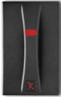
XF1560 Wall-Mount Contactless Smart Reader
